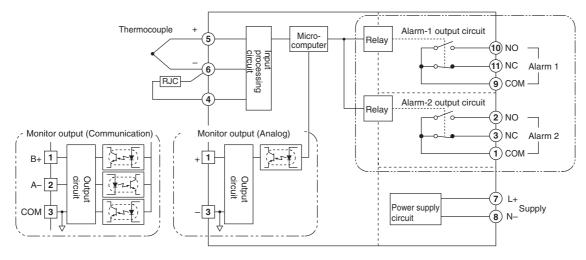
Note: The numbers in "O" indicate the terminal numbers of socket.
