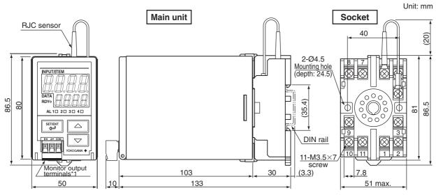
\*1 To be added when the monitor output is specified.
